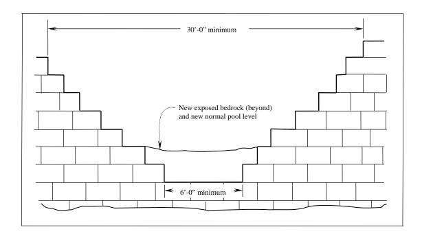
As seen in the photograph on the preceding page, the downstream face of the dam has lost a number of stones over the years. The proposed V-shaped notch would lie in the area of this structural loss.
