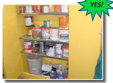
These paint containers are stored indoors in a closeable storage unit, separated by waste type. Their labels are intact and readable.
